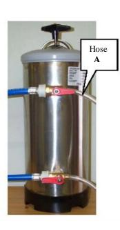
To add salt move the top red lever 180°, water will start running out of pipe A. Wait until the water has stopped running.
